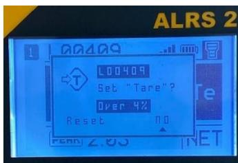
To remove the tare and zero enter the tare mode and select reset.
