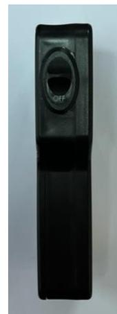
To switch the ALRS2 handset on press the power button
