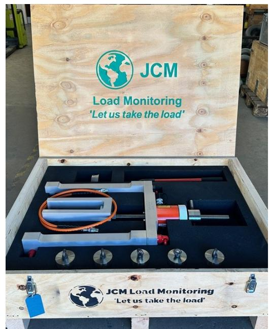
Our 30 Tonne pad eye tester is capable of testing pad eyes from 9.5—30 Tonne.
