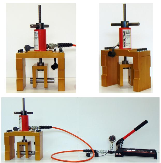
Following on from the success of our 25 Tonne pad eye tester we decided to design and build a 10 Tonne pad eye tester.
